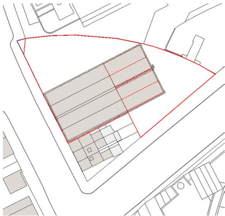
Figure 125 – demolition plan for 12 Pymont Street
